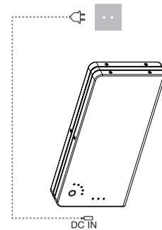
Use the power adapter and connect it to mPowerpack 180 at the port marked 'DC IN'. Plug the power adapter into the wall socket.
