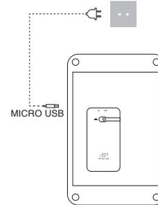
Connect mPowerpad 2 Go to the wall socket using the USB cable (micro USB to the port marked 'IN') and a USB power adaptor\*. Once connected it will start charging.
