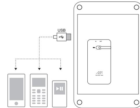
To charge your phone and other electronic devices, connect it to mPowerpad 2 Go's 'OUT' port using the device's USB cable. Once connected, the device will start charging while the LED indicators will light up. As the charge level in the solar charger decreases, the number of lighted LEDs will also decrease. When mPowerpad 2 Go is completely out of charge, no LEDs will be lighted up.
