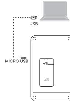
Connect mPowerpad 2 Go to the computer using the USB cable (micro USB to the port marked 'IN'). Once connected it will start charging.
